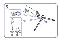
Relaxation fasten the connecting screw at the bottom of the stand base.
