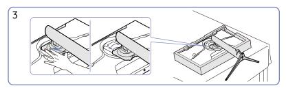
Hold the release bottom and the stand pull down in the direction of the arrow.
