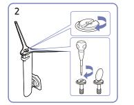
Tightly fasten the connecting screw at the bottom of the stand base.
