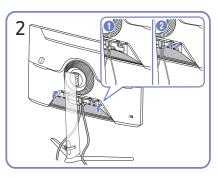
Arrange the cables against the bend tendency of the cables and pull the cables out of the COVER-REAR SUB grooves.
