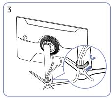
Put both cables in the cable holder on the stand (HOLDER-STAND CABLE) to organise the cables, as shown in the figure. Assembly is complete.
