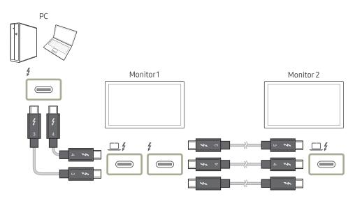
Dual display (daisy chain) support depends on your PC and the connected Thunderbolt™ 3 / 4 cable. The Thunderbolt™ 3 port on your PC must support dual 4 K @ 60 Hz output, and the particular 40Gbps Thunderbolt™ 3 / 4 cable (☐ ▼ ○ □, ☐ ▼ □) need to be purchased separately. For detailed specification of the Thunderbolt™ 3 / 4 cable, visit the official Thunderbolt website.
