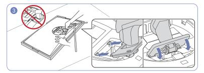
Place the protective Styrofoam (cushion) included in the package on the floor and place the product facing down on the Styrofoam, as shown in the image.
