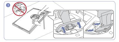
Unfasten the 2 screws at the bottom of the stand Lift and remove the stand in the direction of the arrow as shown in the figure.
