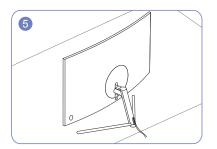
Fasten the screws at the bottom of the stand neck. Tide up the connected power supply and the data cable then cover the COVER-REAR SUB as shown in the figure.
