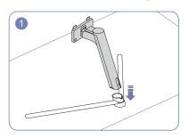
Insert the stand neck into the stand base in the direction shown in the figure.
