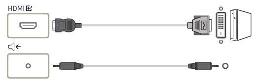
The audio function is not supported if the source device is connected using the HDMI-DVI cable.
