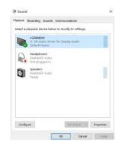
If the USB cable and the HDMI or DP cable are connected from monitor to the computer, two speakers named LS24A40xV and Speakers (LS24A40xV) respectively from the monitor will show in the Sound setting interface. The difference between LS24A40xV and Speakers (LS24A40xV) is only different signal source. You can choose either one to set as the default speaker for monitor.
