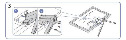
Place a soft cloth over the table to protect the product and place the product onto the cloth so that the front of the product is facing downwards. Push the assembled stand into the main body in the direction of the arrow as shown in the figure. Tightly fasten the connecting screw at the bottom of the main body.
