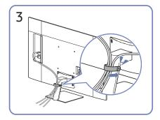
Put both cables in the cable holder on the stand (HOLDER-STAND CABLE) to organize the cables, as shown in the figure. Assembly is complete.
