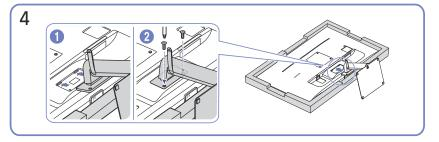
Push the assembled stand into the main body in the direction of the arrow as shown in the figure. Tightly fasten the connecting screw at the bottom of the main body.
