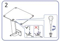
Tightly fasten the connecting screw at the bottom of the stand base. Fasten the large screw in the middle for assembly.
