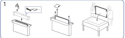
As shown in the figure, remove the product and foam cushion, and then place the product on the table with its front side facing the floor.
