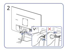
Pull the right side of the HOLDER-STAND CABLE to remove from the stand. The right side of the cable can be damaged when pulled forcibly.
