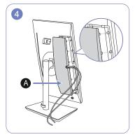
Arrange the cables through the groove on the back of the product, and then attach the COVER-REAR SUB (A). When you attach the COVER-REAR SUB (A), please aim six ribs of the COVER-REAR SUB (A) to the back of the product at first.
