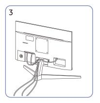
Put both cables in the cable holder on the stand (HOLDER-STAND CABLE) to organize the cables, as shown in the figure. Assembly is complete. Connect the corresponding cables.
