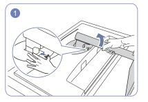
Place the product on a clean and flat floor as shown in the figure. Push the key upward and hold. Turn the stand neck of the display counterclockwise for 10°.
