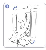
Rotate the machine to the horizontal position.
