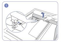
Place the product on a clean and flat floor as shown in the figure. Push the key upward and hold. Turn the stand neck of the display counterclockwise for 10°.
