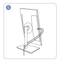
Arrange each of the two cables through either side of the COVER-STAND CABLE, as shown in the figure.
