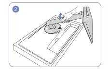
Lift the stand neck in the arrow direction to detach itUnfasten the connecting screw at the bottom of thefrom the display.stand base, and then remove the stand neck from
