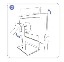
Rotate the machine to the highest vertical position.
