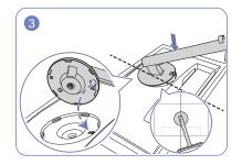
Place the stand neck on the display, as shown in the figure. When you place the stand neck, ensure that the raised button on the display can be inserted into the groove of the stand neck.
