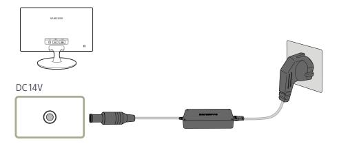
The input voltage is switched automatically.
