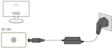
The input voltage is switched automatically.
