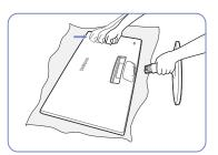
While holding the stand neck with one hand, pound the other fisted hand down onto the top of the stand base in the direction of the arrow to detach the stand base.
