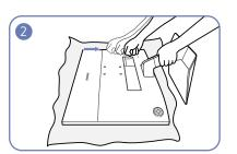
While holding the stand neck with one hand, pound the other fisted hand down onto the top of the stand base in the direction of the arrow to detach the stand base.
