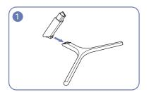
Insert the stand neck into the stand base in the direction shown in the figure.
