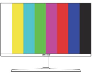
Never turn off the power nor change the input source during self diagnosis. If possible, try not to interrupt testing.
