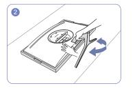
To disassemble the stand from the monitor, be sure to press the lower part of the monitor with one hand, and shake the stand from side to side with the other hand to make some gap between them.
