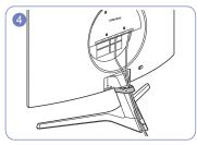
Secure the HOLDER-CABLE to the stand. (HOOK type)
