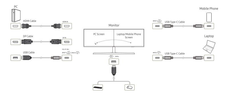
The KVM (keyboard, video, and mouse) switch enables users to use only a keyboard, a video monitor, and a mouse for controlling multiple input sources. The function of the Samsung USB switch is as follows:
