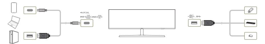
If multiple devices are connected to a source device, the many cables around the source device may look messy. Connecting the devices directly to the product will resolve such inconvenience. Connect a mobile device such as an MP3 player or smartphone to the product connected to a source device. This allows you to control the device or charge the device battery from your PC.
