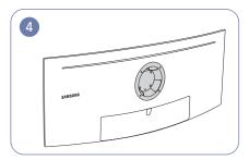
A Attach the BRACKET WALL here
