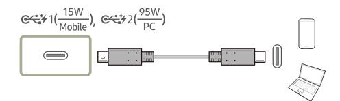
The USB Type-C port can support USB Power Delivery, Data, and DP video signal.
