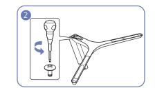
Turn the connecting screw at the bottom of the stand base to separate it.
