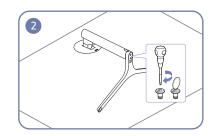
Check that the stand neck is firmly connected. Tightly fasten the connecting screw at the bottom of the stand base.
