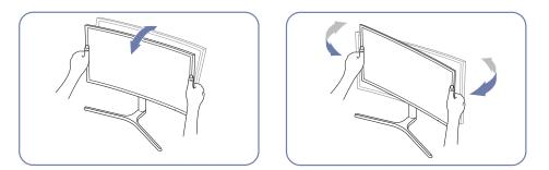
• Grasp the left and right sides of the monitor and adjust the tilt.
