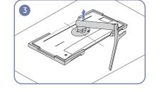
counterclockwise for 10°, lift the stand neck to detach it from the device.
