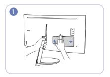
Grab the stand with one hand and use the thumb on your other hand to remove the COVER-REAR-SUB in the direction of the arrow.
