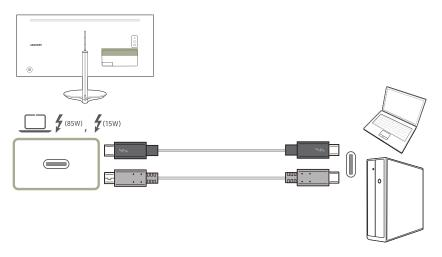
Connect the Thunderbolt  $^{\text{IM}}$  3 cable or USB Type-C cable to  $\bigcirc$  on the back of the product and  $\bigcirc$  on the PC.
