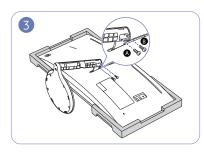
Rotate A and B screws for fixing.
