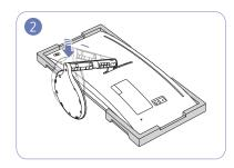
Attach the stand to the back of the monitor, in the direction of the arrow.
