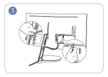
Connect cables to the appropriate ports.
