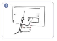
Ensure that the length of the cables, within the range indicated in the image, is at least 170 mm, so that the cables are loose.
