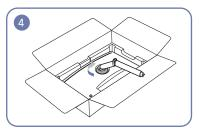
Turn the COVER-REAR TOP clockwise to attach it to the rear cover.
