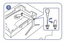
Place the screen on the Styrofoam or soft cushion included in the package, hold the stand base with one hand and remove the screws of the stand base with another hand.
