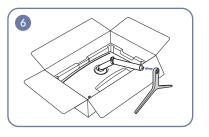
Attach the stand base to the neck, as shown in the image. Make sure there is no gap between the stand neck and base.
