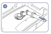
Remove the COVER-REAR TOP after detaching it from the rear cover.
