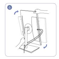
Rotate the machine to the horizontal position.
