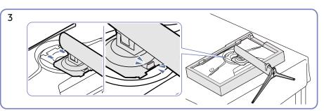
Push the assembled stand into the main body in the direction of the arrow as shown in the figure.
