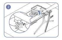
Push the key upward and hold. Turn the stand neck After turning the stand neck of the display of the display counterclockwise for 10°.
