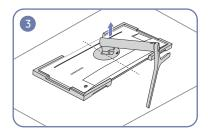
counterclockwise for 10°, lift the stand neck to detach it from the device.
