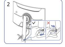
Pull the right side of the HOLDER-STAND CABLE to remove from the stand. The left side of the HOLDER-STAND CABLE can be damaged when pulled forcibly.
