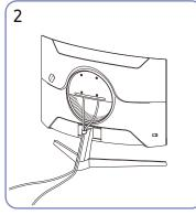
Put both cables in the cable holder on the stand (HOLDER-STAND CABLE) to organise the cables, as shown in the figure. Assembly is complete.
