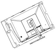
2. While keeping the release button pressed, tilt the base and slide it out.
