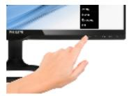
SmartTouch controls are intelligent, touch sensitive icons that replace protruding buttons. Responding to your lightest touch, SmartTouch controls, for example, power up your monitor or brighten and sharpen your display with SmartImage Lite. When activated, SmartTouch icons glow to indicate that your commands have been implemented.
