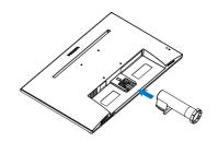
Hold the monitor base stand with both hands and firmly insert the base stand into the base column.
