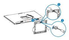
3. Remove the hinge cover from monitor body by using your fingers.
