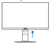
Place the monitor face down on a smooth surface. Pay attention not to scratch or damage the screen. Then lift the monitor base.
