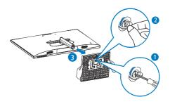
3. Remove the hinge cover from monitor body by using your fingers.
