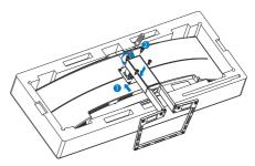
3. After attaching the base, erect the monitor with both hands on holding the monitor together with styrofoam firmly. Now you can pull out the styrofoam. Notice this monitor is curved design, when you pull out the styrofoam, do not squeeze the panel to avoid broken panel.
