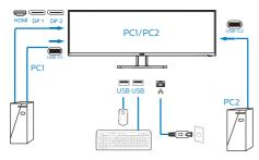
3. Enter to OSD menu. Go to KVM layer and select "Auto", "USB-C1" or "USB-C2" to switch the control of peripherals from one device to another. Simply repeat this step for switching the control system using one set of peripheral.
