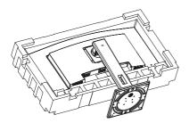
2. While keeping the release button pressed, tilt the base and slide it out.
