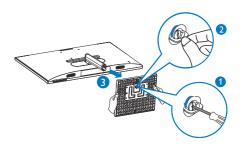
Remove the hinge cover from monitor body by using your fingers.
