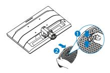
3. Remove the screw from hinge cover.
