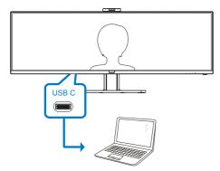
3. Enter to OSD menu. Go to KVM layer and select "Auto", "USB C" or "USB up" to switch the control of peripherals from one device to another. Simply repeat this step for switching the control system using one set of peripheral.
