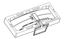
2. Loosen the assembly screws, then detach the neck from the display.
