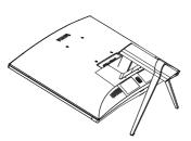
2. Use a screwdriver to remove the screws on the arm, and then detach the arm/stand from the monitor.
