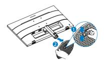
3. Remove the screw from hinge cover.
