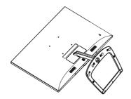
Use your fingers to loosen the screw located at the bottom of the base, and remove the base from the stand
