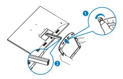
3. Remove the hinge cover from monitor body by using your fingers.
