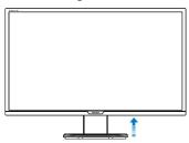
Place the monitor face down on a smooth surface. Pay attention not to scratch or damage the screen. Then lift the monitor stand.
