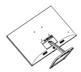
Use your fingers to loosen the screw located at the bottom of the base,and remove the base from the stand.
