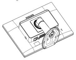
2. Remove the screws from hinge cover.
