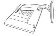
3. While keeping the release button pressed, tilt the base and slide it out.
