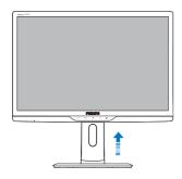
Place the monitor face down on a smooth surface, taking care to avoid scratching or damaging the screen. Then lift the monitor stand.
