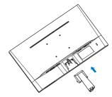
Hold the monitor base stand with both hands and firmly insert the base stand into the base column.
