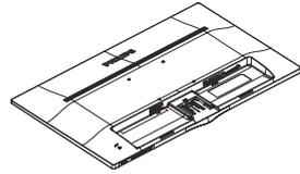
2. Press the locking clips to detach the base stand away from the base column.
