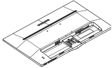
2. Attach the base column with the monitor until it clicks into position.
