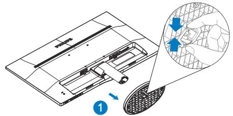
3. Press the release button to detach the base column.
