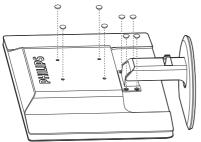
2. Remove the 4 screws and then remove the base from the monitor.
