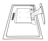
2. Remove the 4 screws and then remove the base from the monitor.
