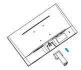
3. Hold the monitor base stand with both hands and firmly insert the base stand into the base column.
