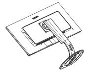
2. Loosen the assembly screws, then detach the neck from the monitor.
