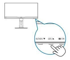
For example, if you selected [Input] as the hotkey, press the USER button on the front bezel, the [Input] menu appears.
